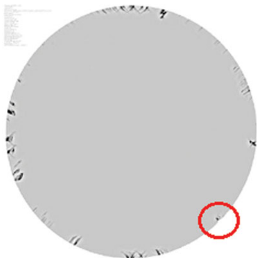
Figure 6. BedeScan™ transmission XRD Image of 200-mm plateau annealed Si wafer at 1000 °C for 30 s showing slip bands developing from the edge. Scan time 0.3 h.
