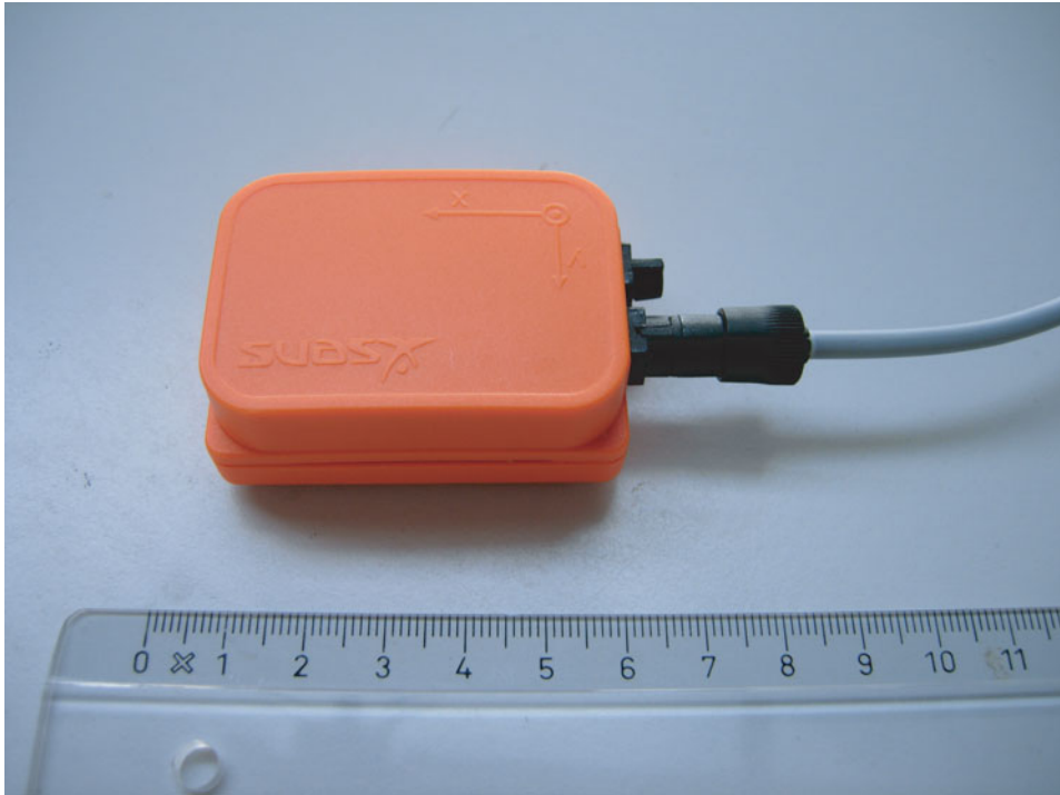
Figure 1. Inertial measurement unit composed of MEMS from Xsens company.
