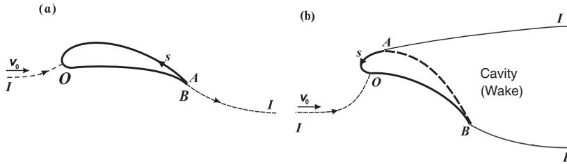
FIGURE 1. (a) Continuous flow over an aerofoil. (b) Helmholtz–Kirchhoff flow with an infinite cavity past a profile.
