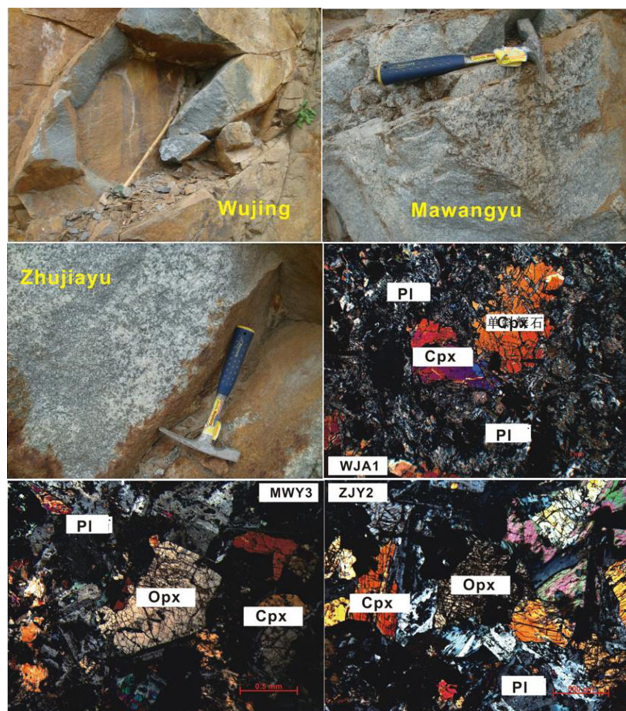
Fig. 2. (Colour online) The field and microscopic photos of the mafic dykes studied. PI – plagioclase; Cpx – clinopyroxene.
