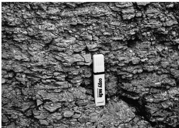
Figure 4. Brecciated Oxford Clay bedrock, exposed in vertical section ~0.4–0.6 m below the base of fluvial gravels at Cleveland Farm Quarry, Ashton Keynes, in the Upper Thames basin; 2 June 1995. 12-cm-long pen for scale.
