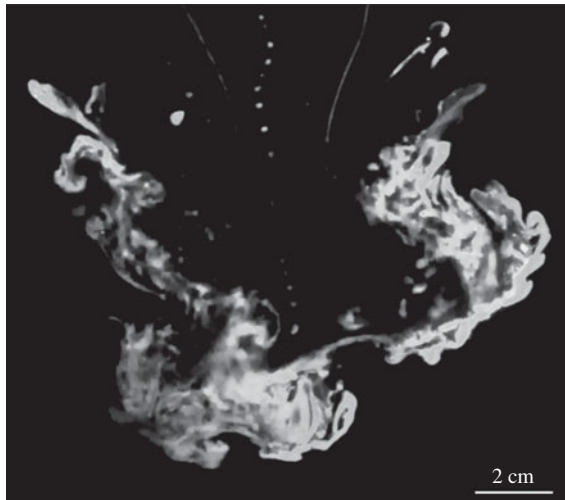
FIGURE 12. Cross-section of an immiscible turbulent thermal, obtained using light-induced fluorescence, modified from Deguen et al. (2014). We \approx 10^3 , P \approx 0.54 , Immersed, z \approx 4R .
