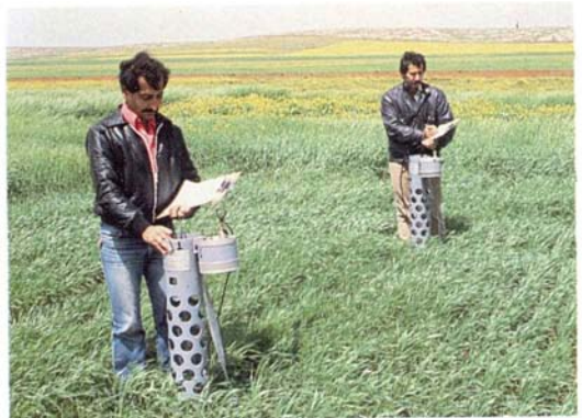
3d. Detailed crop water use studies using neutron probes have been undertaken in NW Syria to assess the effect of phosphorus and nitrogen fertilizer on the water balance of the system.
