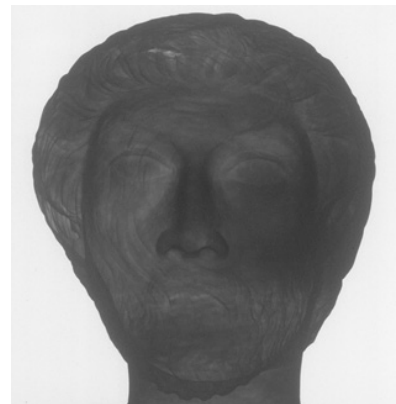
Fig. 3. Overview of the gold bust using X-rays from the source running at 200 kV. Details of the structure and material distribution can hardly be distinguished due to the strong attenuation of the beam and the low transmission (E. H. Lehmann, Paul Scherrer Institut)
