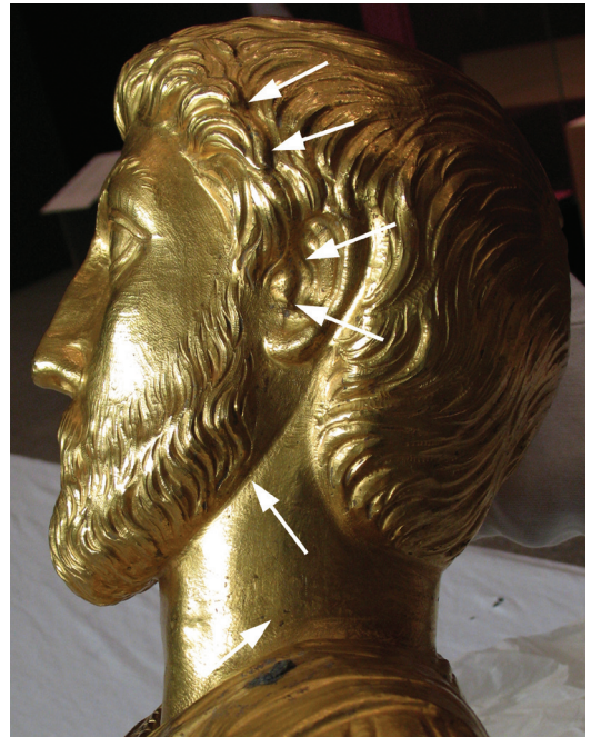
Fig. 12. Tomography of Marcus Aurelius. The arrows indicate small daubs of solder applied on holes and cracks produced by intensive working on the metal structure (E. H. Lehmann, Paul Scherrer Institut).
