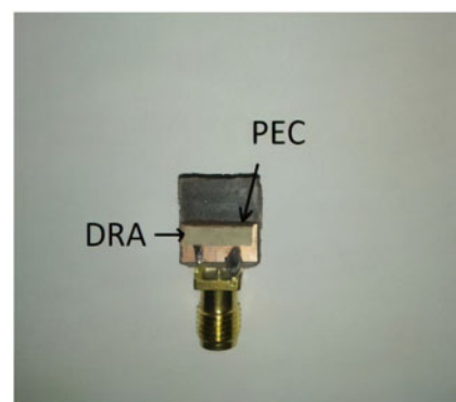
Fig. 7. Prototype of the proposed antenna.
