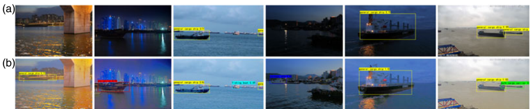
Figure 12. Vessel detection experiments on real low-visibility maritime images. From top to bottom: the vessel detection results on (a) low-light images and (b) enhanced images obtained by LVENet, respectively.
