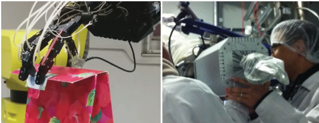
Fig. 9. Practical configurations of the metamorphic hand. (a) Origami carton folding experiment. (b) Dexterous deboning experiment.
