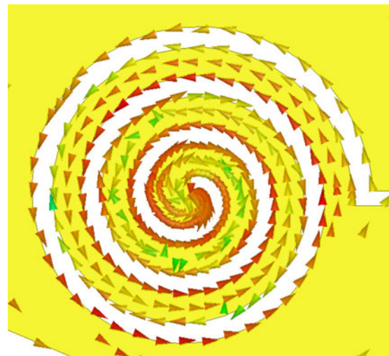
Fig. 5. Surface current around the spiral-slot of the proposed antenna at the notch frequency.
