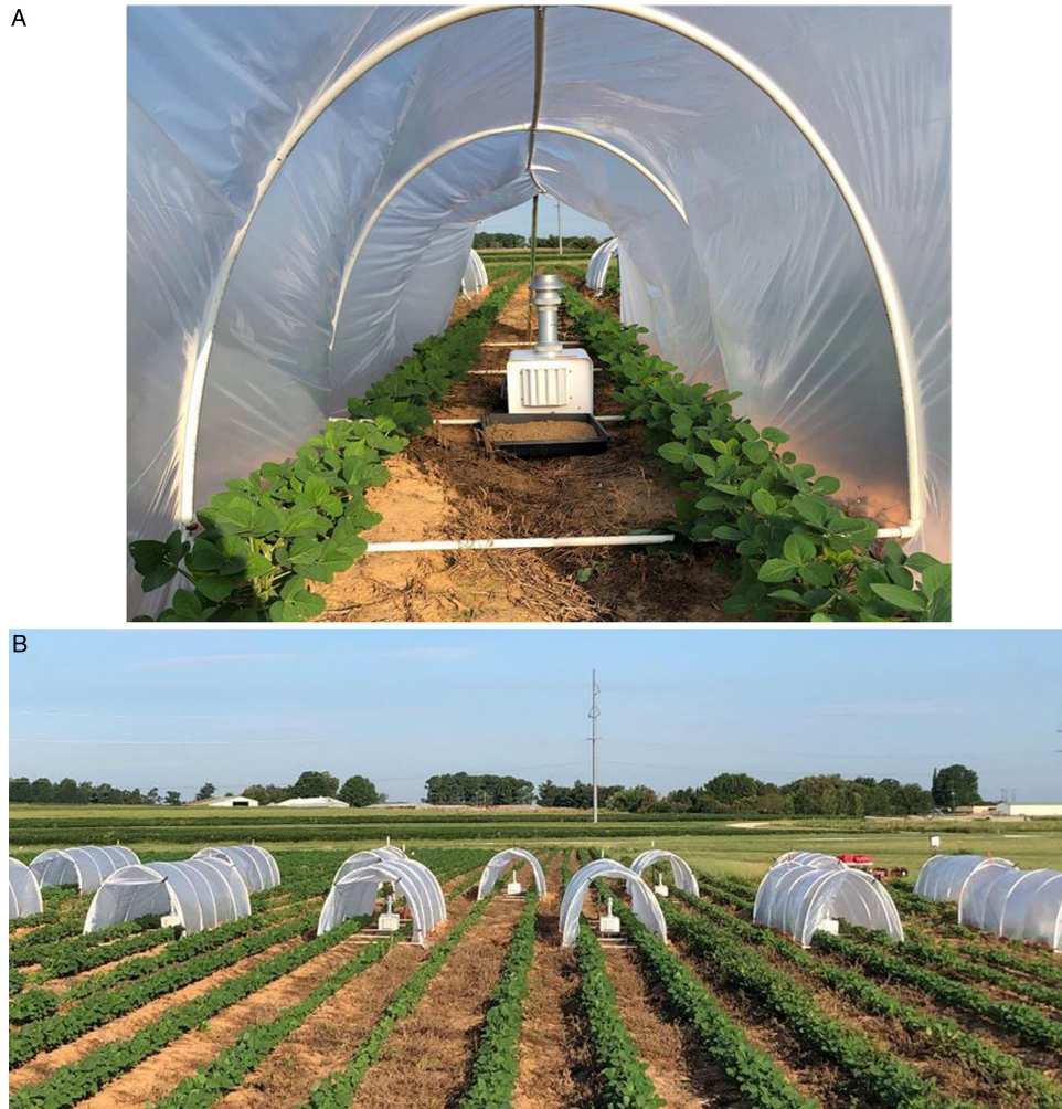
Figure 1. Photos showing a close-up view of the high-volume air sampler and treated trays positioned at the center of the low tunnel (A); and the bottom side view of the tunnels in the field of dicamba-susceptible soybean (B) at the Milo J. Shult Agricultural Research and Education Center in Fayetteville, AR.
