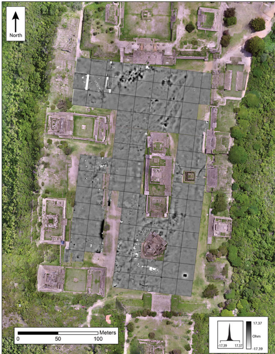
Figure 6. Electrical resistance results superimposed over orthophoto of Main Plaza. (Color online)
