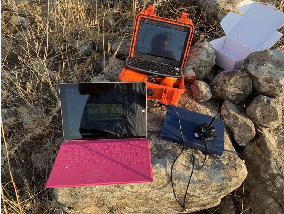
FIGURE 8. Photo showing the rugged computer (in back) running the controller software, and the Surface Pro tablet running QGIS with the hedgehog plugged in via USB. (Photo by A. C. Hill, courtesy of the Galilee Prehistory Project).
