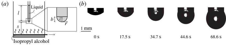
FIGURE 1. (a) A schematic of the experimental apparatus to measure the liquid–gas interfacial tension at different concentrations of IPA vapour. (b) Images of a swelling water drop as the IPA vapour concentration increases with time. The distance of the IPA source to the liquid drop, s , and the initial liquid column height, l , are 20 and 35 mm, respectively.
