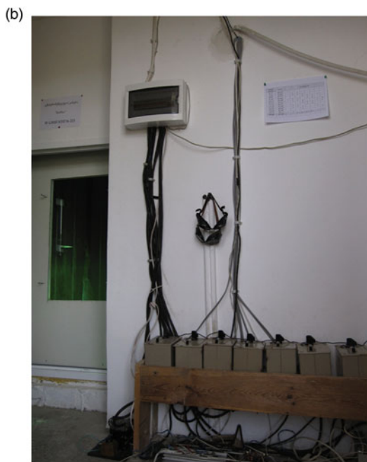
Fig. 1. (a) General schematics of the MCSC 'Artificial Mars': MCSC is a double-coated chamber 15 m 3 in volume, equipped with climate-imitating and measuring tools; Remote semi-automated operation is maintained by the electric-scheme and the supporting computer programmed in accordance with the preliminary calculations. (b) External view of the MCSC 'Artificial Mars': Main circuit block – A and eight start-up blocks for the lamps' ignition – B are visible.
