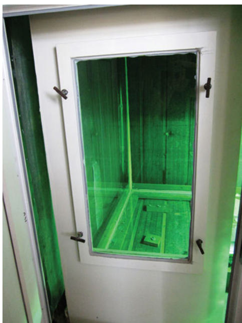
Fig. 4. The inner site of the IVC door and outer site of the entrance are coated by strips of vacuum-rubber that ensures solid attachment on both sides. Every possible empty space and all attached surfaces of the EFC and IVC are filled with low-temperature resistant vacuum-silicate.
