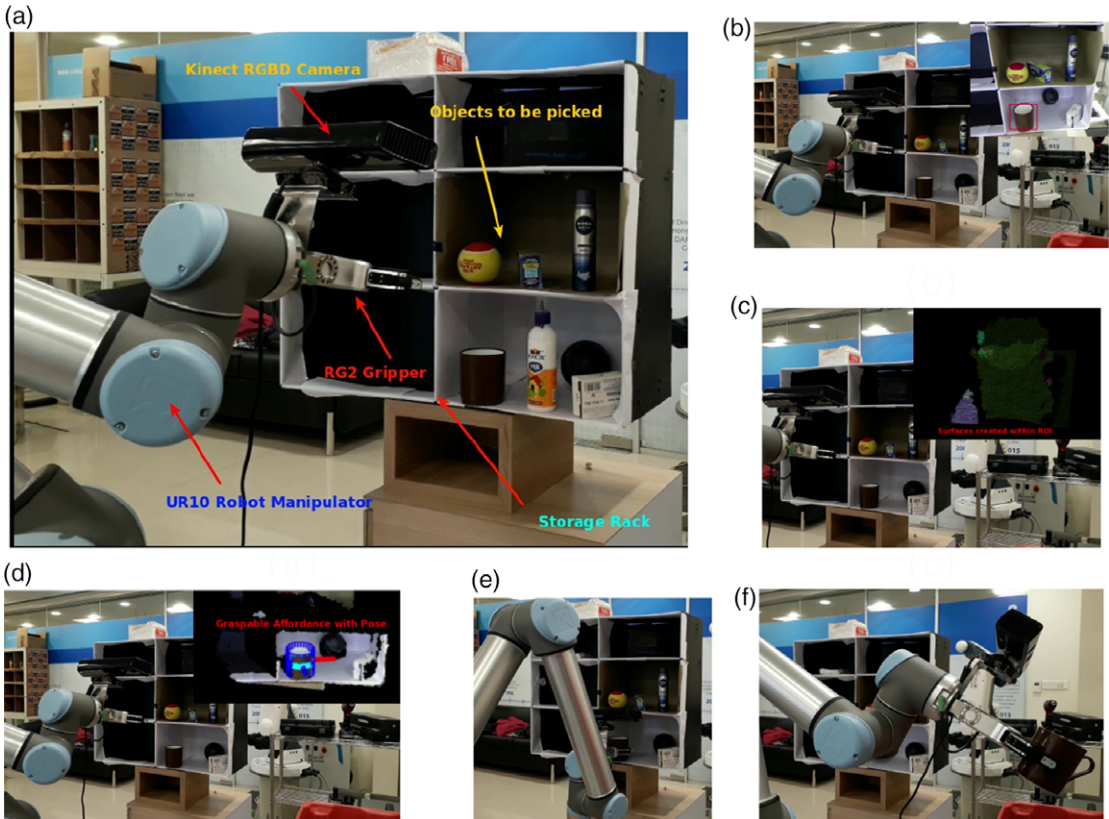
Figure 12. Experimental setup for testing the proposed grasping algorithm. It uses a hand-mounted Kinect camera for perception and a RG2 two-finger gripper for grasping. (a) Experimental setup, (b) object detection using RCNN, (c) surface segmentation within the ROI, (d) primitive shape identification and pose detection, (e) robot motion for grasping and (f) dropping of object into a tote.
