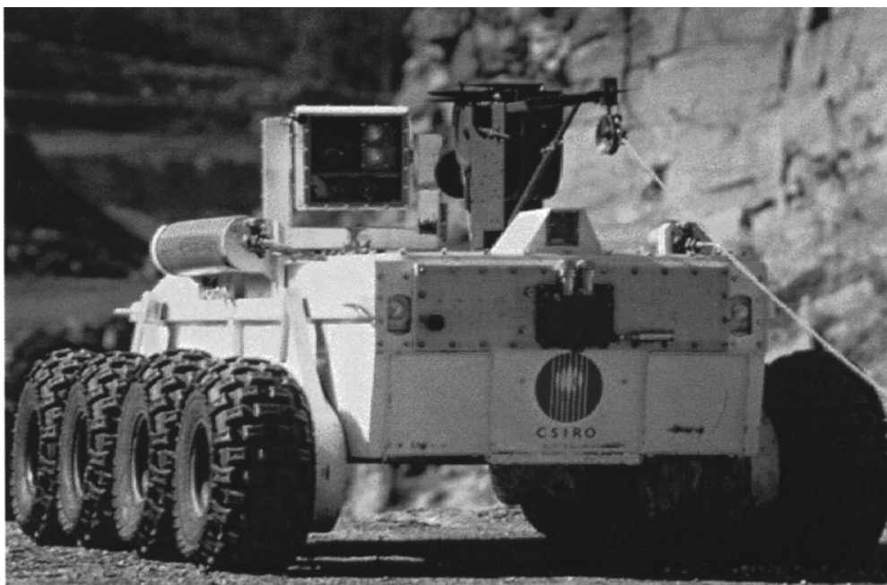
Fig. 17. The Numbat mine emergency response vehicle.
