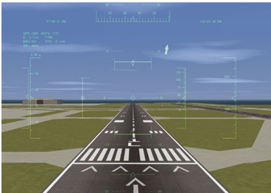
Figure A5. PilotStation out-the-window display with heads-up display.
