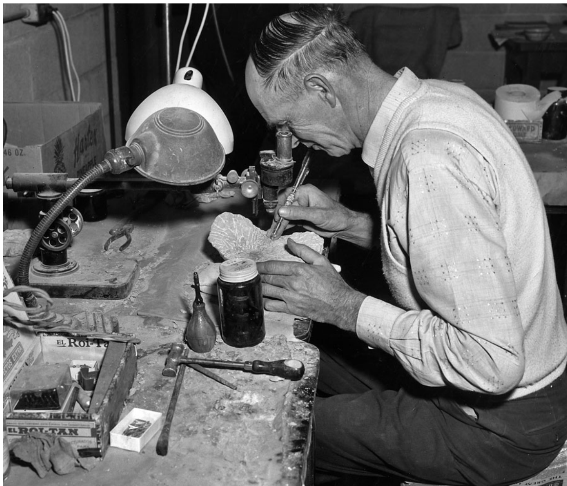
Figure 8 Lansing Craig, preparator at the University of Texas at Austin Vertebrate Paleontology Laboratory in the 1950s. Visible in this photo is a Zeiss XB stereoscopic microscope, a pneumatic airscribe, several types of adhesive, a hammer, chisel, brushes and other hand tools common to nearly every palaeontology laboratory.
