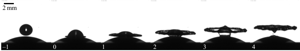
Figure 4. Time-lapse images showing the formation of a non-distinct bubble after impact of a water drop. The label of a frame indicates the time in milliseconds, where t = 0 corresponds to the moment of impact. In the last frame, the bursting of the bubble is visible. The drop with R = 1.33 \text{ mm} impinges at u_l = 1.26 \text{ m s}^{-1} (corresponding to We = 57.4 ) onto the membrane at gas velocity u_g = 3.83 \text{ m s}^{-1} (corresponding to \Delta p_c / (2\gamma/R) = 23.3 ).
