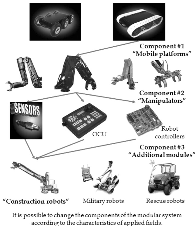
Fig. 2. Framework of a multipurpose field robot.
