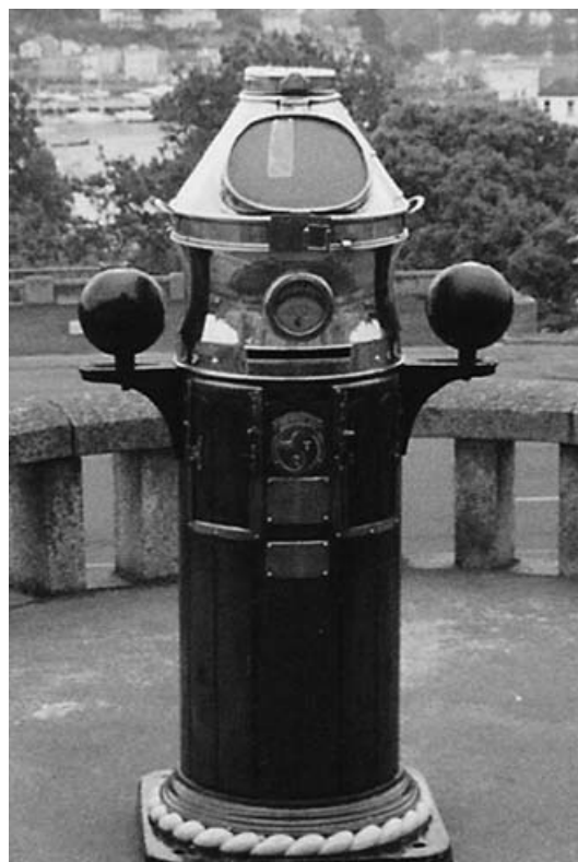
Fig. 4. Binnacle and standard compass of the SS Terra Nova on the Bridge, Britannia Royal Naval College, Dartmouth. Courtesy of the Commodore.
