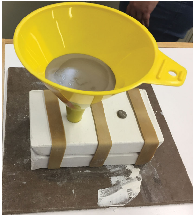
FIGURE 6. Mold being filled with porcelain slip. Note the air hole at the right in between rubber bands.
