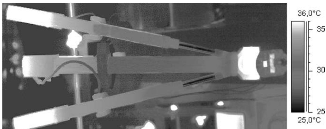
Fig. 10. Thermographic image of Tricept SRT60 after three hours in use.
