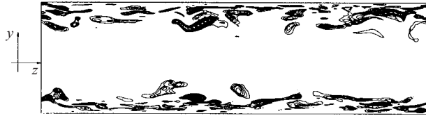
FIGURE 7. Contours of the instantaneous P_{e,t} normalized by u_{\tau_0}^3/\delta for We=8 . Here only negative values of P_{e,t} are drawn for clarity and contour levels are from -1 to -30 .
