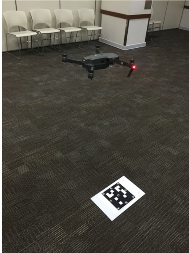
Figure 7. Real UAS landing experiment with MVPN technique in indoor environment (DJI Mavic Pro).
