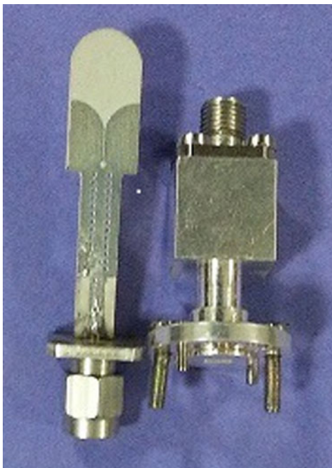
Fig. 5. ETS antenna with elliptical dielectric loading.
