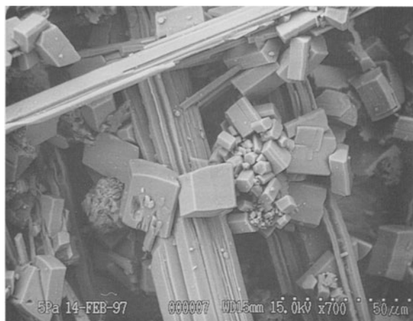
Figure 1. Euhedral crystals of destinezite associated with acicular gypsum from Alum Cave Bluff.
