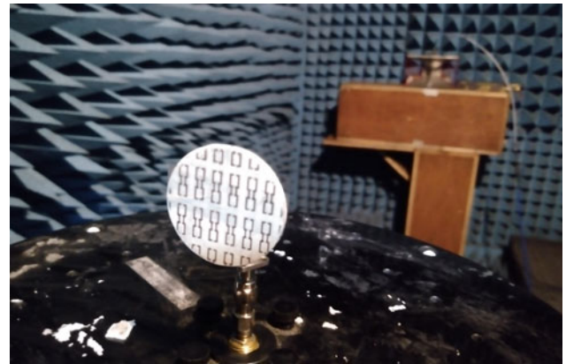
Fig. 14. Designed antenna in an anechoic chamber.
