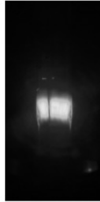
(b) V/N switch works in single-channel mode with pressures of 0.46Mpa in main gap and 0.34Mpa in auxiliary gap
