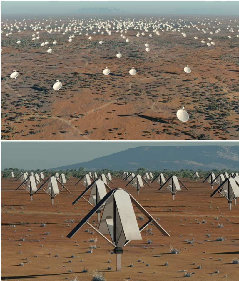
Figure 2. The Phase 1 SKA Observatory will consist of dish and sparse aperture plane array technologies. Two dish antenna arrays, a high-sensitivity array equipped with single-pixel feeds in South Africa will operate up to 3 GHz and a second survey instrument with focal-plane phased arrays in Australia will image large instantaneous fields of view from 0.7 - 1.8 GHz. A separate low-frequency sparse aperture plane array at the Western Australia site, operating down to 70 MHz, will allow sensitive observations of highly redshifted neutral hydrogen emission. (Image credit: SKA Organization/Swinburne Astronomy Productions.)
