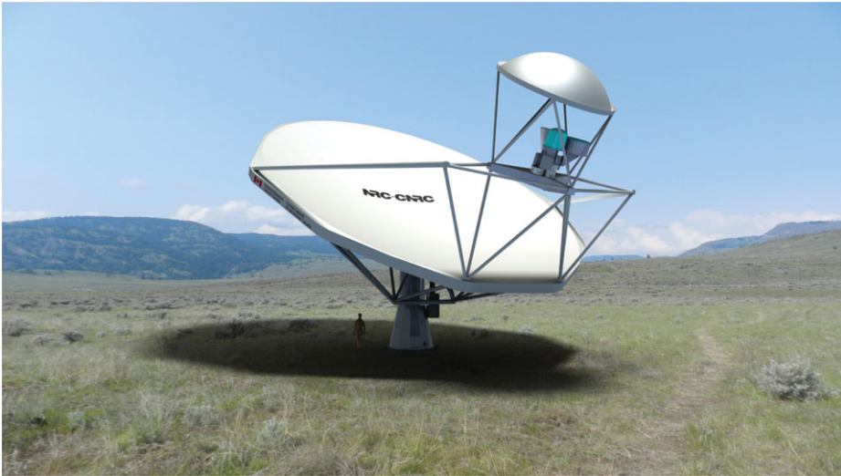
Figure 1. Rendering of a prototype SKA 15-m composite material antenna under construction at the Dominion Radio Astrophysical Observatory in Penticton, Canada. The offset design optimizes for high dynamic range imaging by minimizing radiation scattered into feed. The focal structure will accommodate both single-pixel and focal-plane phased-array feed systems. (Image Credit: National Research Council of Canada, Canada/US-TDP SKA Dish Verification Project)
