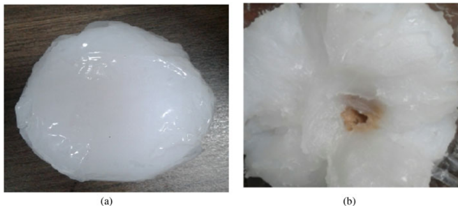
Fig. 11. (a) Breast phantom (b) Tumor made of wheat flour at center of breast phantom.
