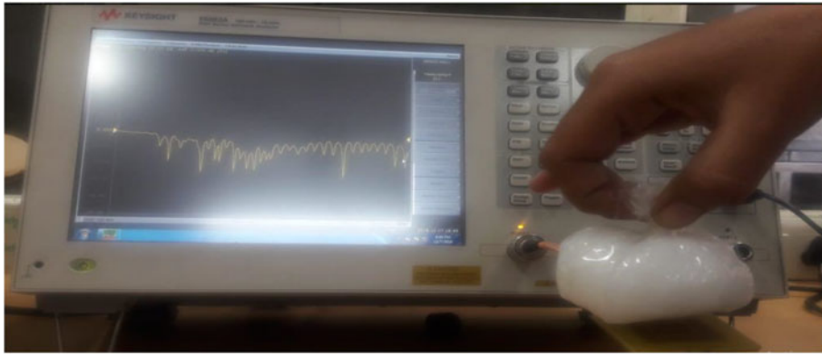
Fig. 12. Measured S parameters of the proposed antenna in the presence of breast phantom.
