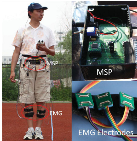
Figure 5. Placement of the EMG sensors and the MSP platform.
