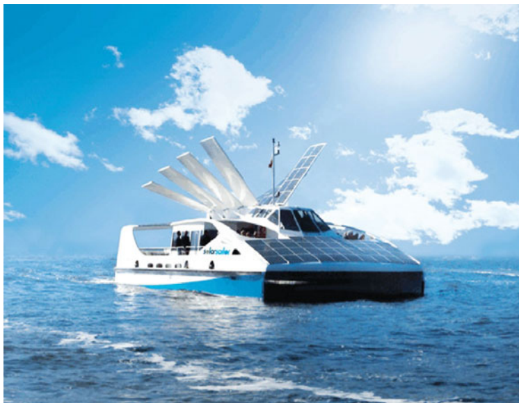
Figure 5. Solar Sailor, catamaran ferry with eight photovoltaic solar panel sails.
