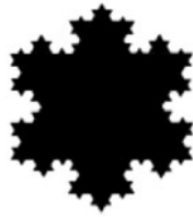
Fig. 1. Koch snowflake: a finite area planar figure which may have an infinite fractal boundary.
