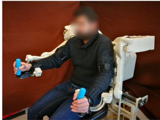
Fig. 1. Master device: the arm light exoskeleton (ALEx).
