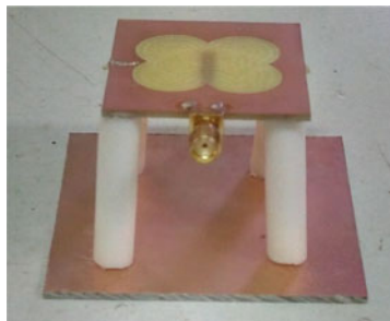
Fig. 7. Side view of the proposed antenna with the reflector.
