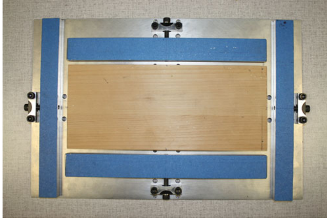
Figure 4. (Colour online) The pre-strain fixture used for adjusting membrane tension.
