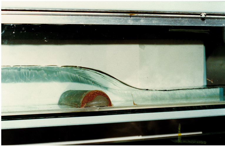
FIGURE 1. A photograph of a critical flow over a semicircular obstacle mounted on the bottom of a horizontal channel.
