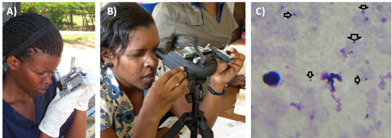
Fig. 1. Familiarization and training of Ugandan Ministry of Health staff in the use of inverted microscopes. (A) An original metal McArthur microscope being assessed; (B) Basic training using the Newton Nm1 microscope on tripod; (C) Digital image of a Giemsa-stained thick blood film (with several malaria parasites indicated by arrows) as taken with an iPhone attached to the Newton Nm1 at \times 1000 (oil) magnification.
