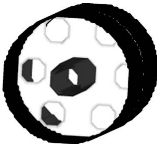
FIGURE 3. Perspective view of a portion (between the inlet and some distance after the baffle plate) of the microreactor. The multi-holed baffle plate is white, while the inner (fuel) and outer (oxydizer) tubes are black.
