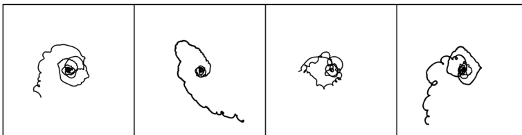
Figure 15. Absolute trajectories of four individual vortices; the size of the square is 6000 \times 6000 (in non-dimensional units), as in panel (d) in figure 14.
