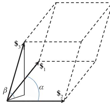
Fig. 2. A parallelepiped spanned by three weighted screws.
