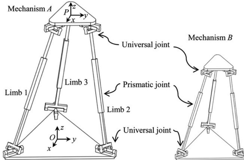
Fig. 3. Two similar 3-UPU manipulators with different sizes.
