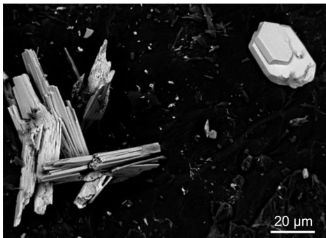
Fig. 2. Back-scatter SEM image of hagstromite (left) and thorneite (right). Fragment from holotype (#73596).
