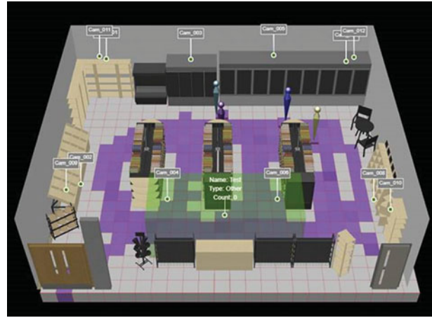
Fig. 4. Illustration of a retail intelligence scenario where multiple cameras are deployed, 3D space is reconstructed, people are detected and tracked, and heatmap (in purple) is generated.
