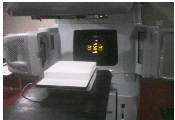
Figure 3. Measurement setup in linac (Varian Clinac iX) where 2D array with solid water phantoms are arranged on the couch.
