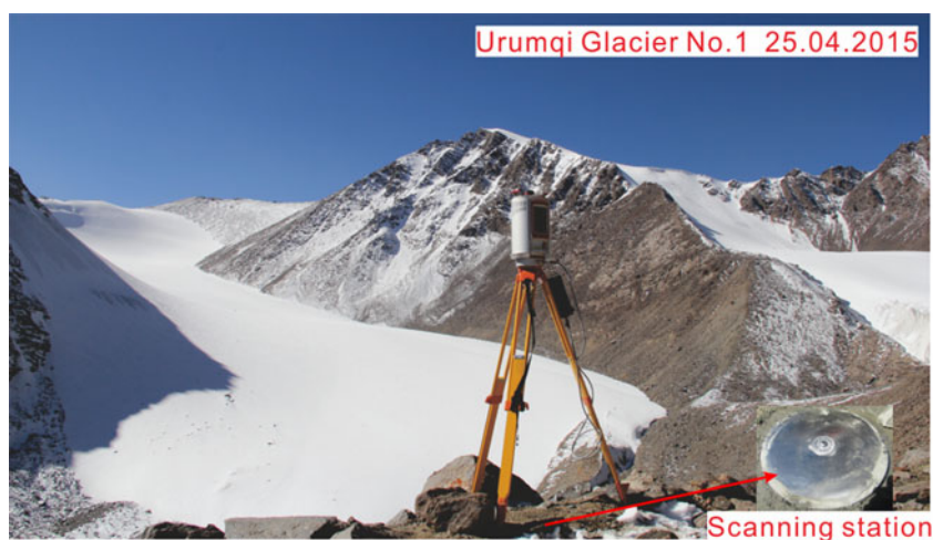
Fig. 2. TLS survey of Urumqi Glacier No. 1 with the Riegl VZ ® -6000 terrestrial laser scanner on 25 April 2015. Lower right corner of the picture was a scanning station, which was fixed using reinforced concrete with a GPS-leveling point.
