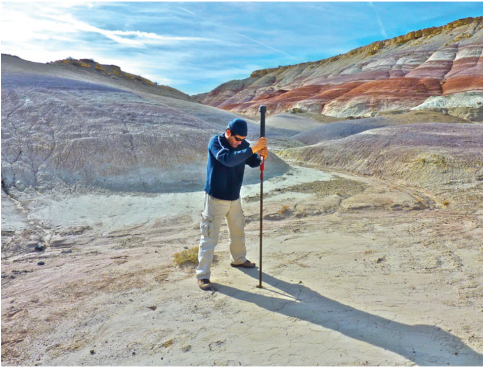
Fig. 5. Collecting a soil core at site S2. The site was in channel fill in between shale hills in the Brushy basin member of the MF. The tool has a sliding weight that is lifted and dropped by the operator, causing an impact that impels the core tube into the soil.
